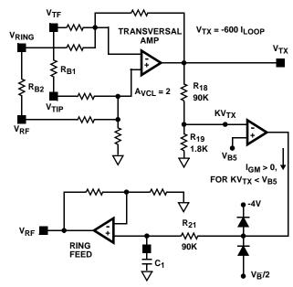
FIGURE 3. DC LOOP CURRENT CHARACTERISTICS
