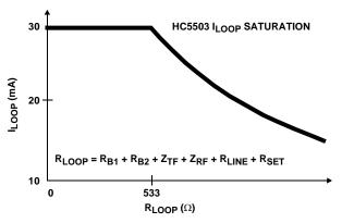
FIGURE 4. DC LOOP CURRENT CHARACTERISTICS
